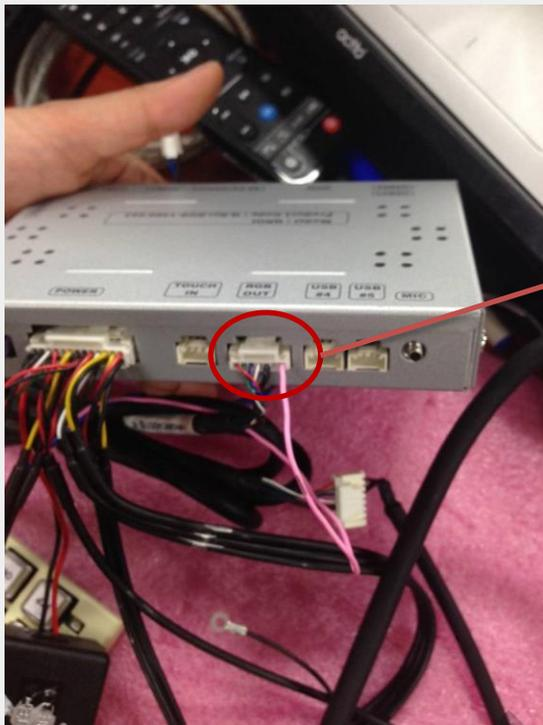
The first pin from the right of RGB Out is Uart wire
