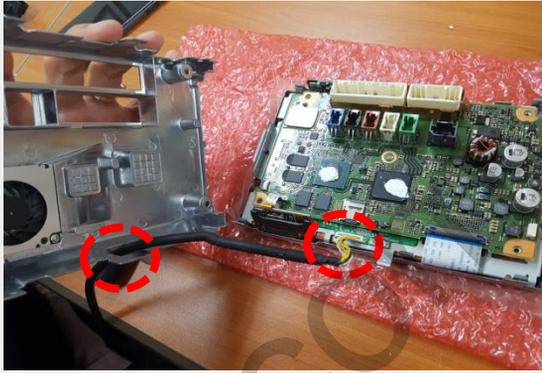
Place the OEM board on the top of the supplied subboard and the other side of the supplied FFC cables is connected as shown above
