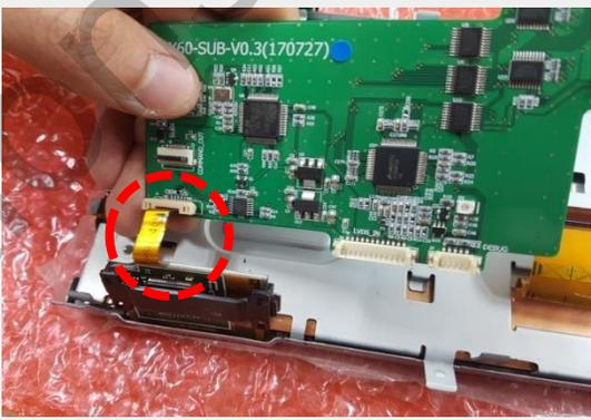
Marked OEM touch cable is connected to "OEM T/S" of the supplied subboard
