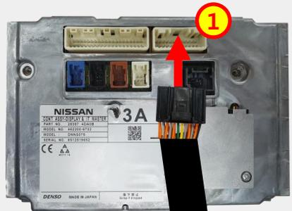
※ Remove the oem cable from the back side of the monitor " 1 " and connect OEM cable to the supplied power cable. Male connector of the supplied power cable is connected to the back side of the monitor
