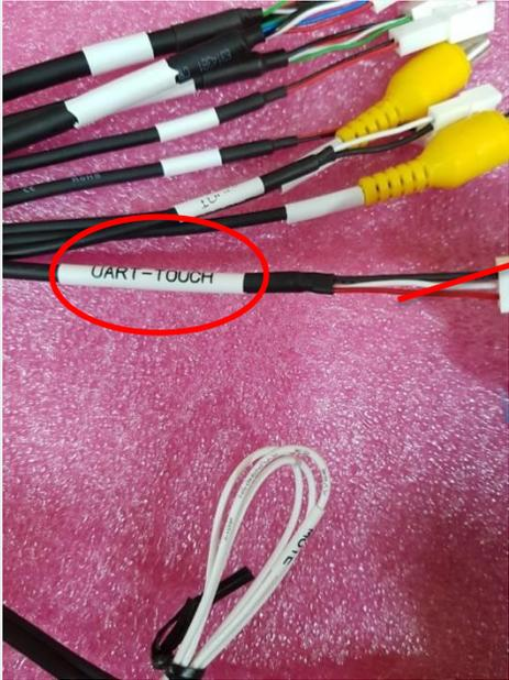
There are three wires for Uart-touch cable from QROI2 multi cable.
