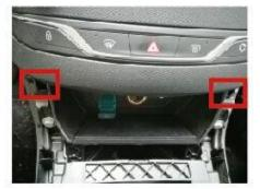
2. Tear apart LCD panel, and take out of Panel of center console
