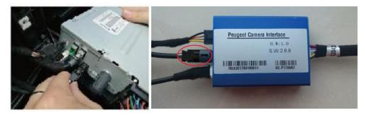
7. Connect camera to camera inputs harness, and finish installation.
