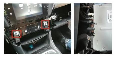
4. Plug out of Quadlock connector, and connect it to Interface cable accordingly.
